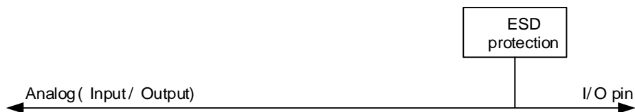
Figure 8-4. Basic structure of Analog configuration
