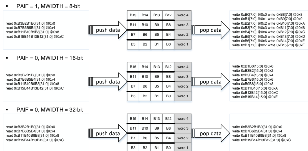
Figure 12-6. Data packing/unpacking when PWIDTH = '10'
