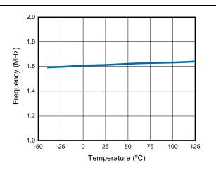
Figure 2. Switch Frequency vs. Temperature
