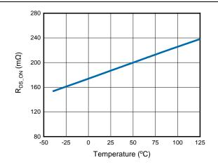
Figure 4. High-side FET ON Resistance vs.
