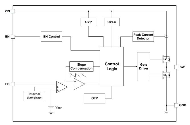
Figure 5. GD30DC1109 Functional Block Diagram
