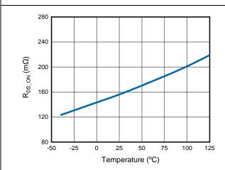
Figure 3. Low-side FET ON Resistance vs.
