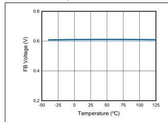
Figure 1. FB Voltage vs. Temperature
