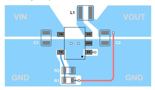
Figure 38. Typical GD30DC1109 Example Layout
