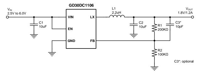
Figure 6. 1.8V, 1.2A Reference Design
