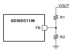
Figure 7. Feedback resistor divider
