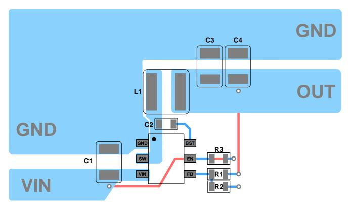
Figure 4. Typical GD30DC1350 Example Layout
