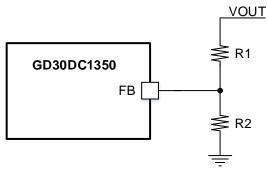
Figure 3. Feedback resistor divider
