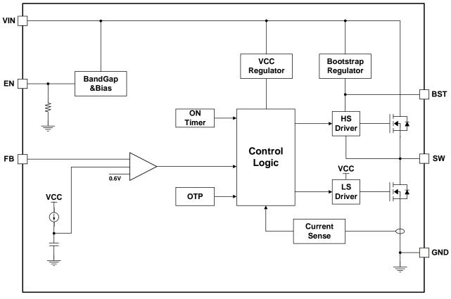
Figure 1. GD30DC1350 Functional Block Diagram
