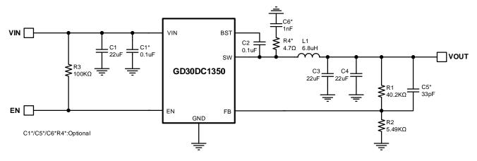
Figure 2. 5.0V, 3A Reference Design
