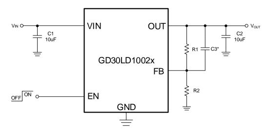
Table 7-1 Adjusted  $V_{\text{OUT}}$  by external feedback resistor
