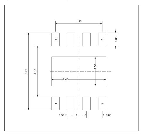
(Original dimensions are in millimeters)
