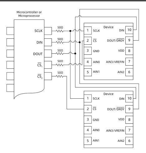
NOTE: GD30AD3641 power and input connections omitted for clarity.
