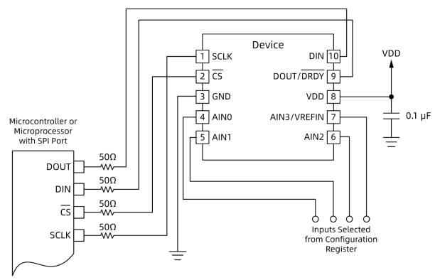
Figure 24. Typical Connections for GD30AD3641
