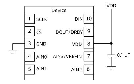
Figure 27. GD30AD3641 Power Supply Decoupling
