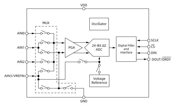
Figure 18. GD30A3641 Block Diagram
