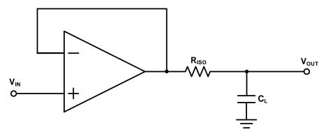
Figure 12. Indirectly Driving Heavy Capacitive Load
