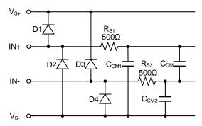
Figure 11. Input EMI Filter and Clamp Circuit
