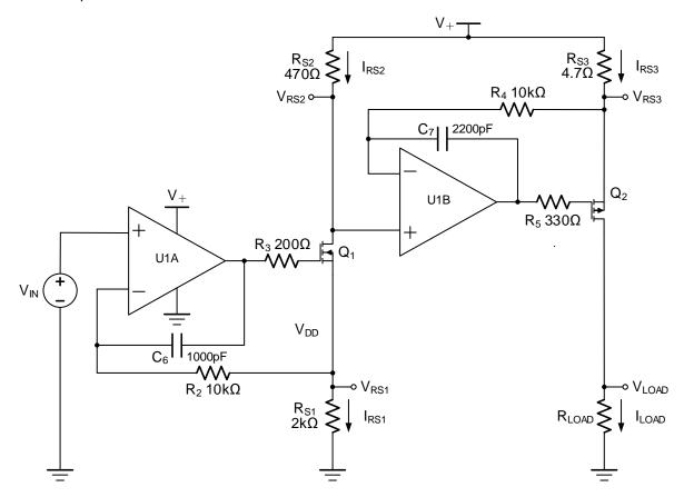
Figure 18. Bidirectional Current-Sensing Schematic
