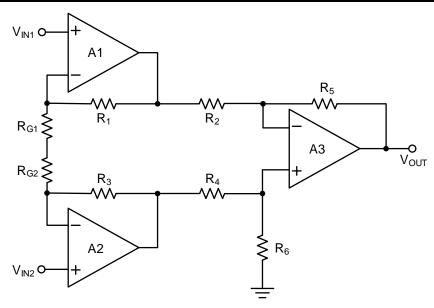
Figure 20. Discrete 3-Op-amp Instrumentation Amplifier
