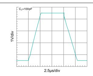
Figure 9. Large Signal Step Response(4V step)
