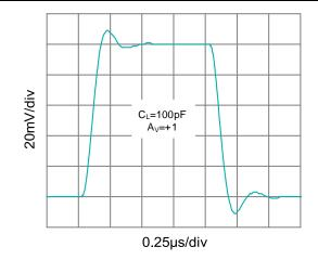
Figure 10. Small Signal Step Response(0.1V step)
