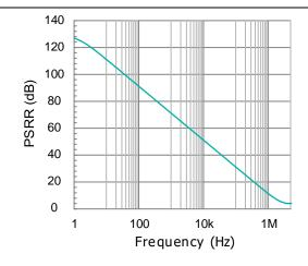
Figure 4. Power Supply Rejection Ratio vs. Frequency
