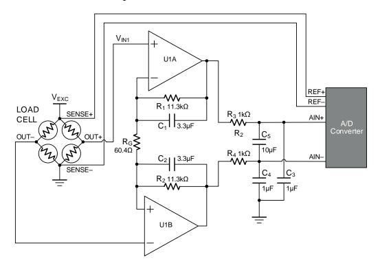
Figure 21. Precision Weigh Scale Measurement System
