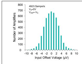
Figure 1. Input Offset Voltage Production
