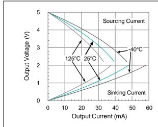
Figure 7. Output Voltage Swing vs. Output Current
