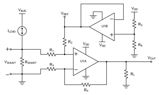
Figure 16. Bidirectional Current-Sensing Schematic
