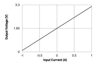
Figure 17. Bidirectional Current-Sensing Circuit Performance: Output Voltage vs. Input Current
