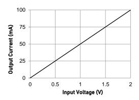
Figure 19. Measured Transfer Function for High-Side V-I Converter
