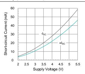
Figure 8. Short-circuit Current vs. Supply Voltage
