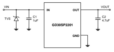
Figure 10. Typical Application Circuit
