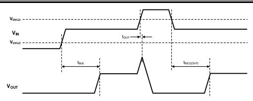
Figure 8. Input OVP Timing Diagram
