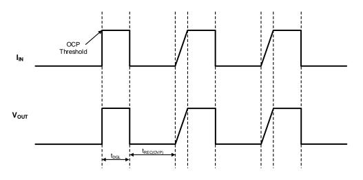
Figure 9. Input OCP Timing Diagram
