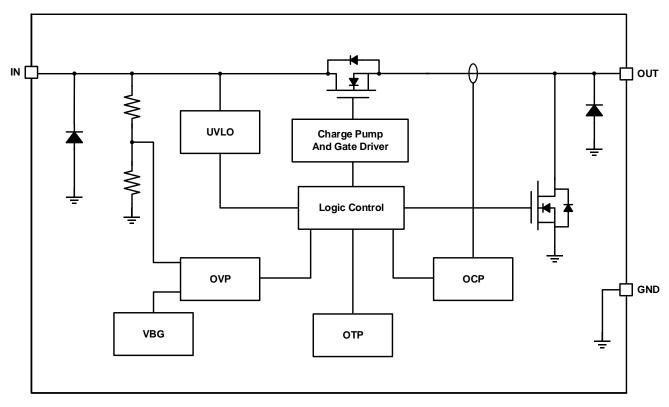
Figure 7. GD30SP2201 Functional Block Diagram
