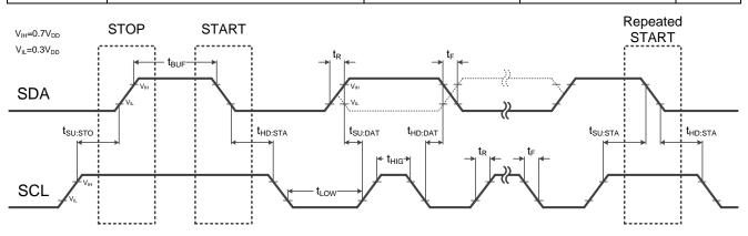
Figure 3. Two-Wire Timing Diagram
