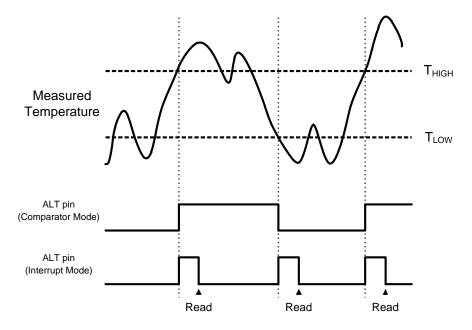
Figure 2. ALT Pin Modes of Operation
