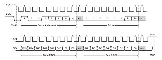
Figure 4. Two-wire Write Command Timing Diagram
