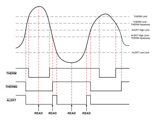
Figure 2. Three Alarm Functions
